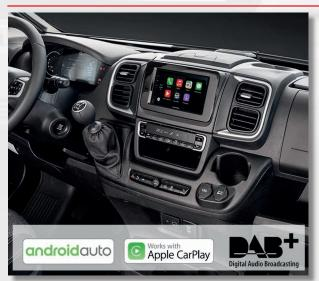
Dedicated installation kit for FIAT Ducato 8 (2021). Supplied with wiring harness with steering wheel control recovery unit and finishing mask.
