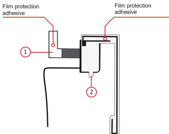
1. Remove the protective film from the foil for mass connection and apply pressure on it to evenly apply the surface to the upright.
